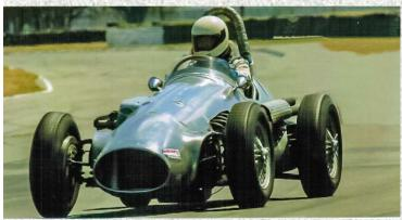
The alloy body was formed in Invercargill by Barry Leitch's company with reshaping the nose and bonnet by Cliff Bennett of Dunedin. Lots of moving parts to this project.
