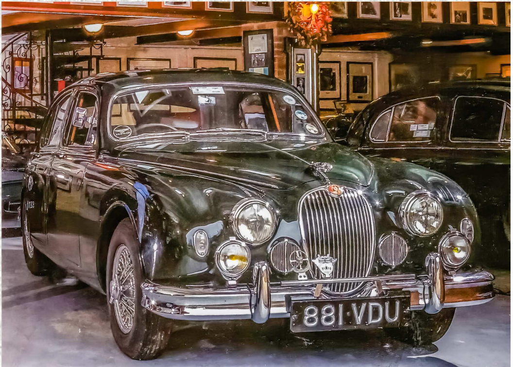
A replica of Mike Hawthorn's Mk 1, 881 V.D.U (3.4l) in British Racing Green on wire wheels, complete with Hawthorns grille badges - mounted on the separate badge bar
