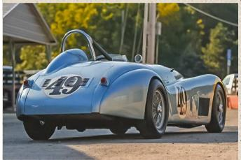
The body is finished in metallic blue with old fashion No. 49 on its flanks. The bumper, headlights and grille have been removed, and a custom wraparound windscreen replaces the old two-piece windshield. Side vents, and a headrest fairing have been added. It is equipped with Dunlop 16- inch tyres and wire wheels with knock off spinners.
