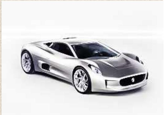
This vehicle was a two-seater, plug in hybrid. It was to produce around 900BHP driving four electric motors, one at each wheel. The most innovative technology was that the batteries driving these motors were to be recharged using two diesel fed micro gas turbines. With this in mind, Tata Motors, invested in a company called Bladon Jets which was near Jaguars headquarters in Coventry.
