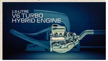
The new car will use the same power unit as 2021 which is a 1.6 litre turbo- hybrid engine which produces the amazing 875Bhp to 1,000Bhp depending on which team one looks at. With such power and very light bodies these cars must feel like they are flying. Top speeds in 2021 were said to be around 400ks an hour.
