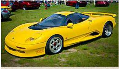
The body work was composed of carbon fibre and Kevlar. It was the first road going car built entirely of these composites, beating the McLaren formula one car by some six months. Total all up weight was 1.050kgs.
