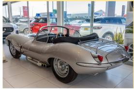
just as they were originally. It was a mammoth undertaking to remake a "new original" version. The result is Michaels magnificent XKSS finished as per the originals. It has a 195 kW (262 bhp) 3.4 litre straight six engine, paired with a four-speed racing Moss gearbox with race clutch. We hope we can hear the throaty roar of this machine.
