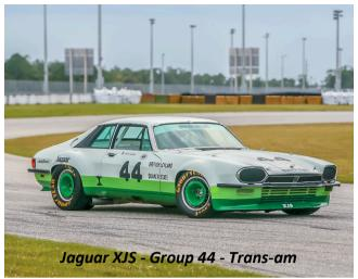
were very much modified. They had of course the mandatory roll cage, race suspension, wider wheels and larger brakes. The V12 engine used a dry sump, 6
