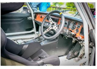
retained the walnut veneer dash and electric windows! The body received flared wheel arches, brake cooling ducts and the body lightened by caustic dipping and a considerable amount of drilling and removal of surplus metal.
