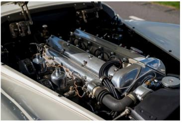
All mechanicals, including matching number engine and gearbox as well as rear axle and brake systems were fully restored. Also forged pistons were installed and many other upgrades to the 3.4 twin cam straight 6 engine. Nice to see a little of New Zealand's history bought back to life again.
