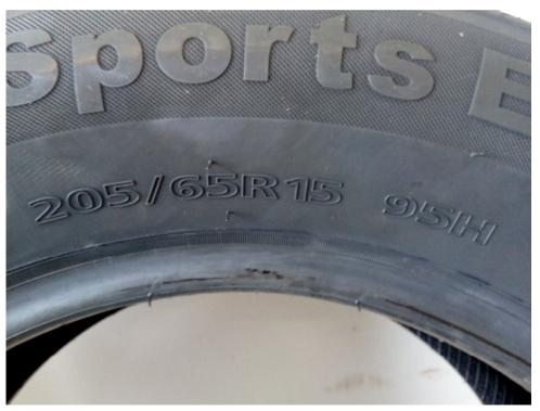
Note; some tyre sizes are in Imperial therefore the diameter and width is shown in inches and are mainly American 4x4 and not relevant to us. The "R" stands for Radial – the construction of the tyre. The "15" is the rim diameter in inches which is a bit unusual in that the rest of the vehicle (relatively new ones) are all made in metric sizing.
