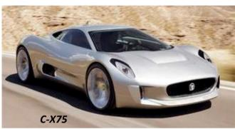
The C-X75 was expected to reach a top speed of 330 kph and a 0 - 62 mph of 3.9 seconds. It was to be powered by 4 x 165 KW (194 hp) electric motors, one on each wheel. Total power was 780 bhp and torque of 1,600 NM. Each motor weighed 110
